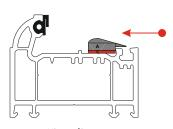
Fit a Frame Wedge "A" to include the packer "C" on the outer frame in the stay fixing area as shown
